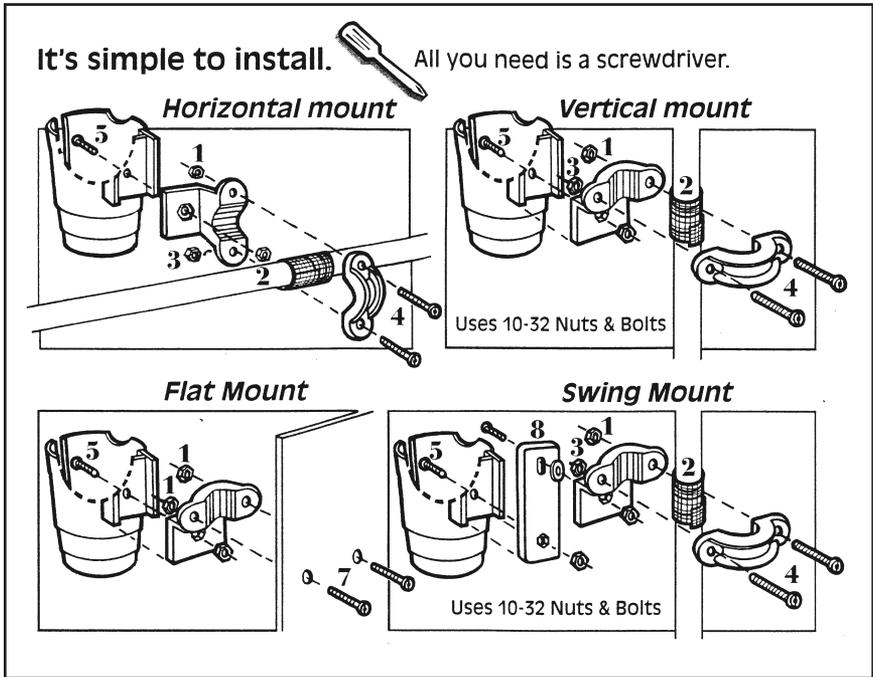
5. Attach the Drink-Aide® container holder to the clamp with the short bolt and nut. Tighten firmly.
